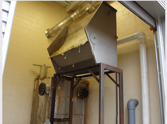
After brewing, solid waste is separated, then sent to a digester to become burnable biogas.
